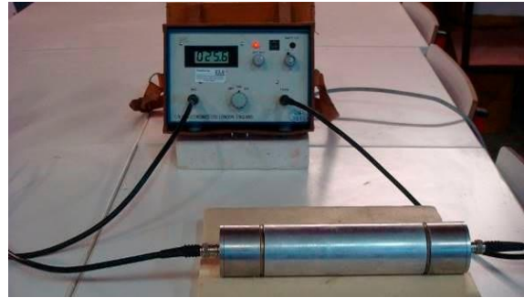
Figure 7. Calibration of the PUNDIT apparatus.
