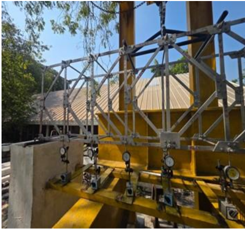
Fig. 4: Experimental loading setup (elevation) showing support conditions and load points.
