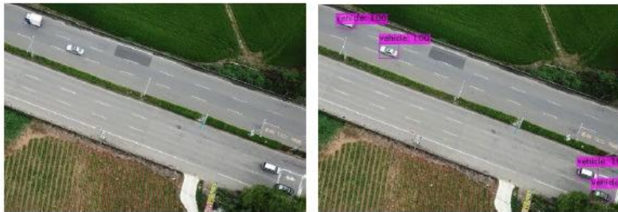
Figure 6 Input image of VAID Dataset (Left Side), Predicted Output Image from the Our Model (Right Side) showing four vehicles
