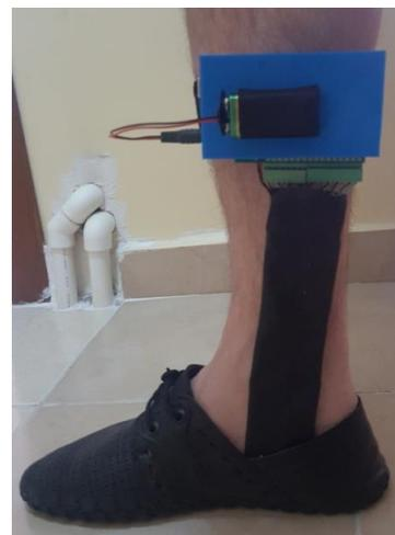
**Fig 12.** Wearable Kinetic IoT System
