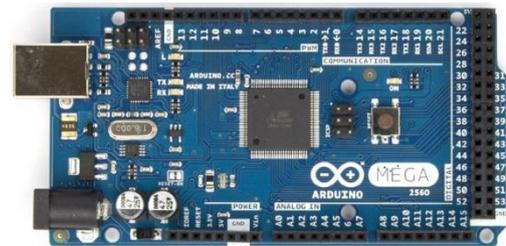
Fig 5. Arduino Mega 2560
