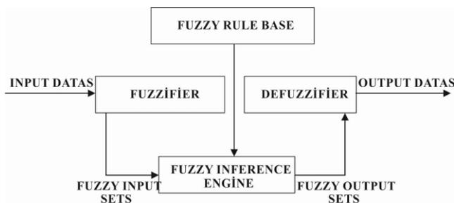
Figure 2. Blurring defuzzification fuzzy system with unit
