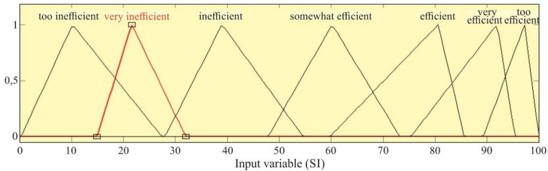
Figure 4. The membership function of soil index (SI)
