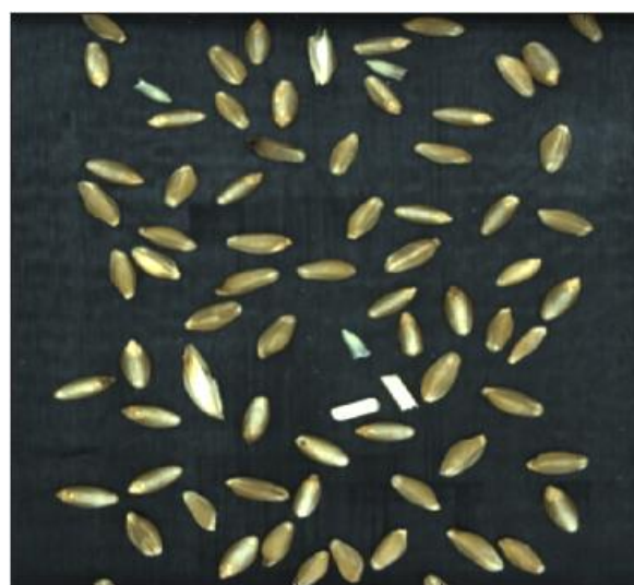
Figure 3. Frame sample of the video visualizing durum wheat grains with impurities
